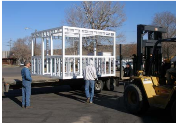
The 12' x 12' framed is unloaded after powder coating
